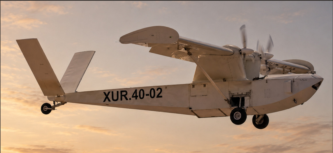
Figure 1. Flyox I in flight — side profile showing high-wing cantilever design and retractable landing gear.
