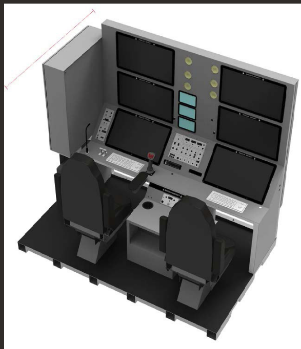
Figure 2. Ground Control Station — the console from which SINGULAR OS operates.
